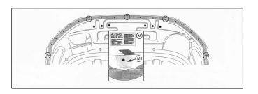
At the five noted locations pull the rubber gasket forward and clean the around the holes in the bonnet with the alcohol wipe.
