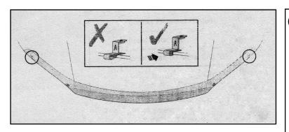
O: Slide the outer push-on metal clips(A) onto the bonnet locating them over the anti-abrasive tape strips as shown.
