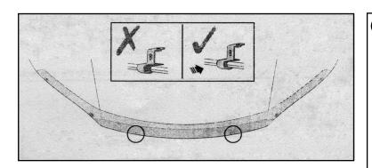
9: Slide the inner push-on metal clips "B" onto the bonnet locating them over the anti-abrasive tape strips as shown IMPORTANT: Ensure that the clips are positioned over anti-abrasive tape and does not come into contact with any of the bonnet's paint work. Failure to do so may result in permanent paint damage.
