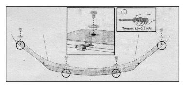
11 : Loosely secure the Bonnet Protector to the four push-on metal clips with the samll screws and fibre washers.
