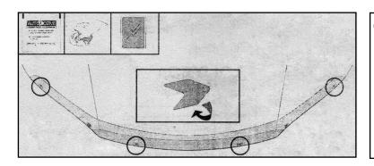
8: At the inner and outer hole locations clean bonnet with the alcohol wipe provided and wipe off any residue with a dry clean cloth Adhere the anti-abrasive tape strips directly below the holes in the Bonnet Protector Apply tape so approximately half of the tape is on the topside and half is on the underside of the bonnet.
