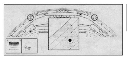
③: Clean the top side and underside of the bonnet at the previously noted areas with the alcohol wipe provided. Wipe off any residue with a dry clean cloth.
