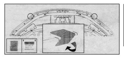
(5):Adhere the anti-abrasive tape strips centered in between the fixed metal clip marks. Apply tape so approximately half of the tape is on the topside and half is on the underside of the bonnet. Clean off the pen marks with the alcohol wipe provided.
