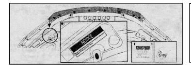
13): Open the bonnet. At the indicated location clean the underside of the bonnet with the alcohol wipe provided and wipe off any residue with a dry clean cloth. Adhere the notice label to the underside of the bonnet.
