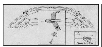
(6):Position the fixed metal clips onto the bonnet and secure the clips by pressing the screw plug through the metal clip into the bonnet.Next insert self tapping screws into the screw plugs, as shown Note: Ensure torque setting 1.5-2.0NM is used.
