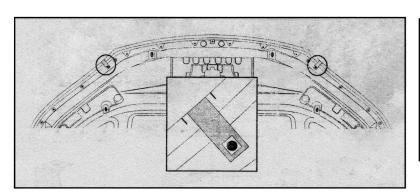
(4):Trial fit the fixed metal clips aligning the rectangular holes in the clips with the previously noted holes in the bonnet. Mark 5mm either side of the fixed metal clips.
