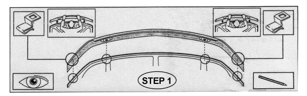
Wash the bonnet with a mild soap and solution, then dry thoroughly. Open the bonnet. Trial fit the Bonnet Protector centrally onto bonnet. With a non-premanent marker, note and mark the positions of the holes in the Bonnet Protector onto bonnet Also note the metal wing clips. Remove Bonnet Protector.
