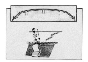
Locate the metal wing clips over the abrasive resistant tape strips on the bonnet lip. Fasten Bonnet Protector with small screws and washers provided. Max torque 0.5Nm TO REMOVE: Reverse above procedure. IMPORTANT: Ensure that the cilps are positioned over abrasive resistant tape and do not come in contact with any of the bonnet's paint work. Failure to do this may result in permanent paint damage.
