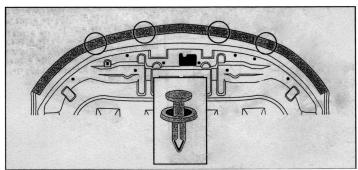
2: Pull the rubber extrusion off the hidden scrivets, remove the four previously noted scrivets and discard.
