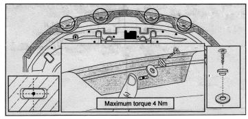
4: Re-install the Hood Protector, ensuring that the collar of the screw plugs locate into the slots in the Hood Protector tags, in the orientation shown. Insert the four self-tapping screws through the plastic screw cap, and nylon washers into the screw plugs, but do not fully tighten.
