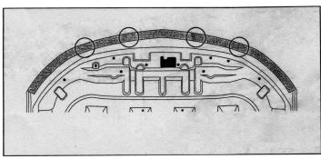
5: Stretch the existing holes in the rubber extrusion over the olastic screw caps.
