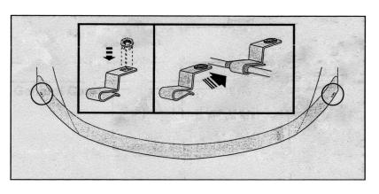
7: Fit the nut insert into metal wing clips. Slide the metal wing clips over the abrasive resistant tape strips on the hood lip.
