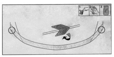
6: Clean the noted areas under the wing clip locations with the alcohol wipe provided. Wipe off any residue with a clean, dry cloth. Adhere the small abrasive resistant tape strips over the hood lip. Apply the tape so that approximately half of each strip is on the top surface of the hood and half is on the underside.
