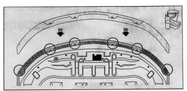
1: Trial fit the Hood Protector centrally onto the hood. With a non-permanent marker or pencil, note the positions of the acrylic tags and the four centre slots in the Hood Protector that correspond with the rubber extrusion. Also note and mark the two metal wing clip locations.
