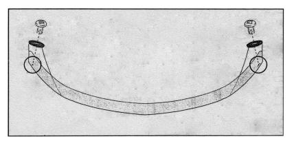
8: Fasten the Hood Protector wings with the screws and small washers provided. To Remove:Reverse above procedure. Note:Check tension of part periodically and tighten screws if required.
