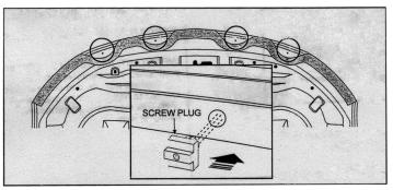
3: Insert the screw plugs provided into the four vacant holes.
