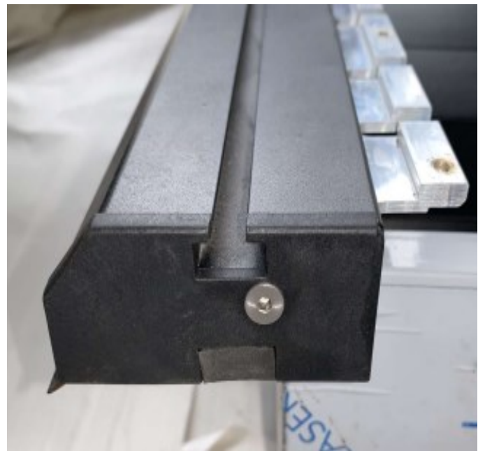
After fixing the horizontal side rail, install the rubber cover of the front end of the side track.
