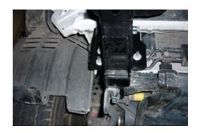
Secure using a modified original lower bumper support bracket as shown.
