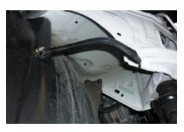
**9.** Drill factory holes out to to 12.5mm and attach chassis bracket using hardware provided and tighten all bolts.
