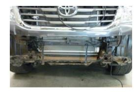
**6.** Remove four bumper support brackets and modify plastic air deflectors as shown.
