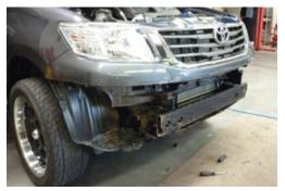
**5.** Remove bumper bar reinforcement.
