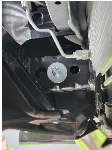
Figure 7: Spacer inside chassis. Figure 8: Bolted through chassis. Figure 9: Two washers.
