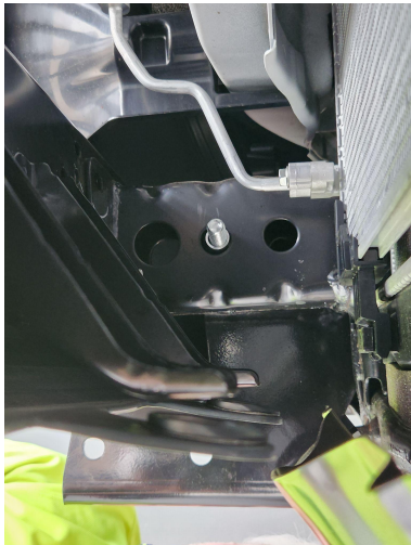
Figure 7: Spacer inside chassis. Figure 8: Bolted through chassis. Figure 9: Two washers.
