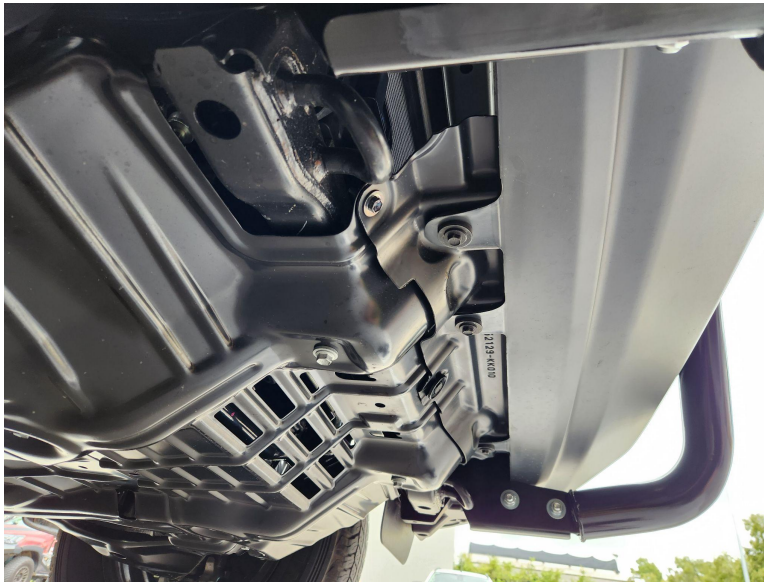
Figure 11: Plastic dust tray re-installed on the vehicle.
