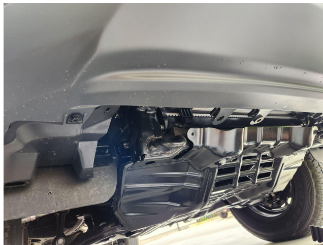
Figure 2: Removed plastic dust cover.
