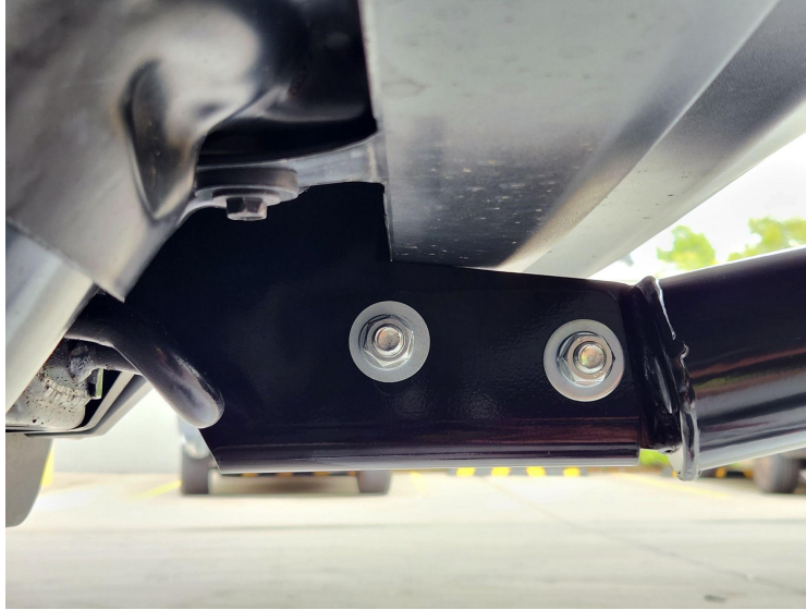
Figure 10: Nudge bar bolted to brackets.
