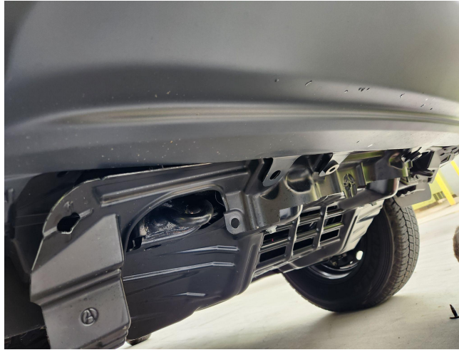
Figure 1: Plastic dust cover with clips removed.
