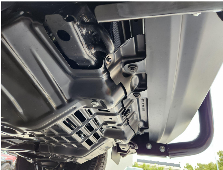
Figure 11: Plastic dust tray re-installed on the vehicle.
