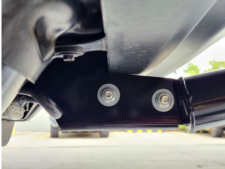
Figure 10: Nudge bar bolted to brackets.
