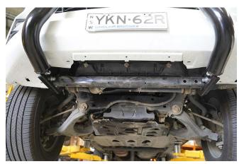
Attach the Black Nudge Bar [2] using M12\*35mm Hex Bolt [8], two M12\*30mm Flat Washers [8], M12 Spring Washers [10] and M12 Nut [12] to the brackets.
