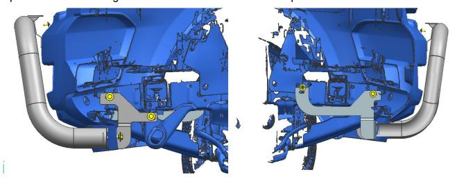
Step 3 (for Ranger PX2 2015-2018): Install the 2 support brackets onto the cross member in front of the radiator. Fix the other side to the side nut-serts of the nudge bar.
