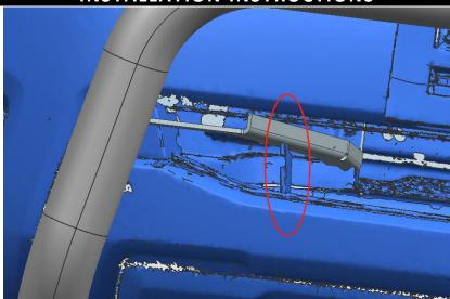
Step 3 (for Ranger PX3 2018-2022): Take the two original bolts on the top of license plate and install it on the top brackets as below picture. Fix the other side to the nudge bar.
