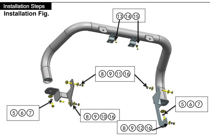
Step 1: Before you start the installation, make sure that you have all the components listed above. Step 2: Fix the left and right brackets to the vehicle as below picture.
