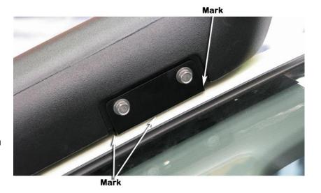
Remove the snorkel body (Item 1) from the vehicle and remove the upper mounting bracket (Item 3) from the snorkel body.
