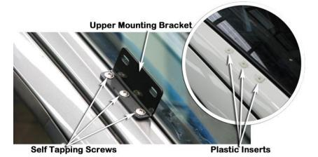
Carefully install the snorkel body (Item 1) to the guard panel, align the snorkel body to the guard panel and upper mounting bracket.
