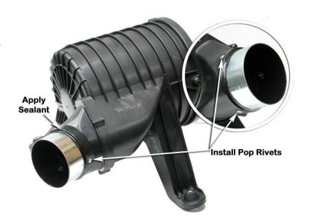
Trial fit the air cleaner housing and check for adequate clearance between the steel adaptor and the standard hole in the inner guard panel, if necessary mark the inner guard panel for the extra clearance.
