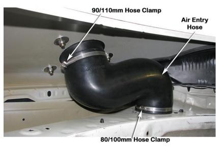
Align the hose for best fitment, correctly position the 80/100mm and 90/110mm hose clamps at either end of the air entry hose and tighten the hose clamps.
