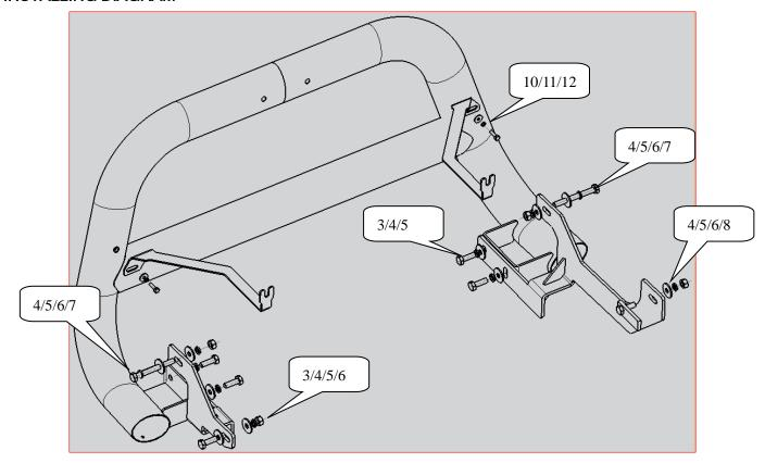
Install the grille guard and brackets to the vehicle follow the installing diagram.
