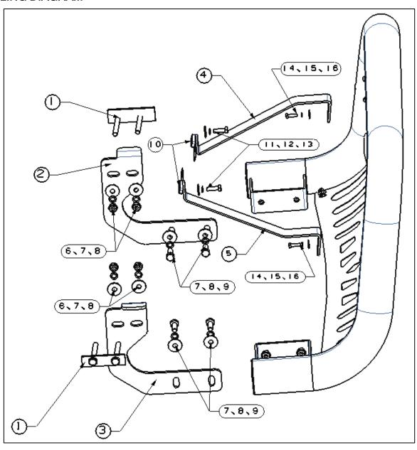
Install the nudge bar and brackets to the vehicle following the installing diagram.
