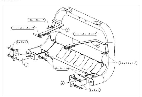
Step 1: Find threaded holes on the chassis under the vehicle as shown in following pictures, and install L&R brackets with (567), do not totally tighten at this step.
