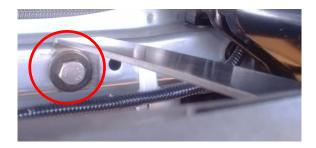
Step 3: Connect the grille guard to the brackets with (890), and to supporting brackets with (150), do not tighten first.
