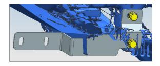
Step 2: Find mounting holes located at the air-inlet grille as shown in following picture, install L&R supporting brackets with (11)(12)(13)(14), do not totally tighten first.
