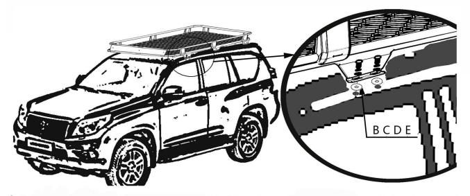
4. Please adjust the roof racks to the best position, tighten all the bolts, the installation is complete.
