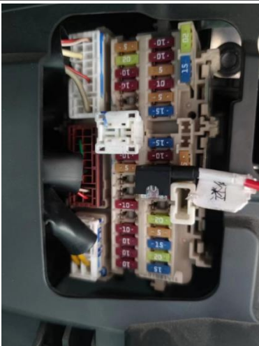
1、 Power positive wiring location
