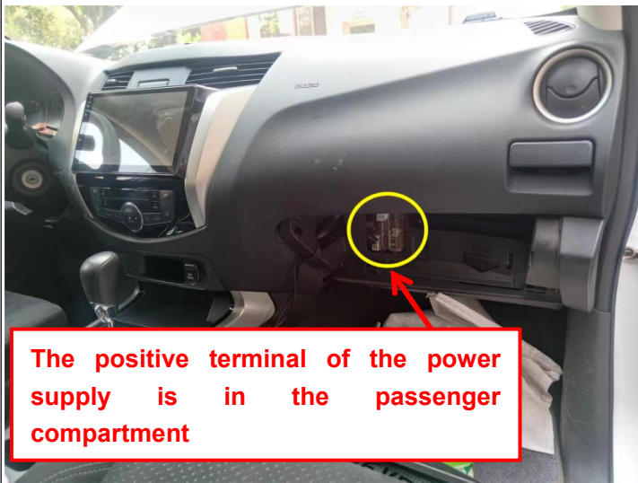
Wiring position of power cable and strapping wire, position of ECU
