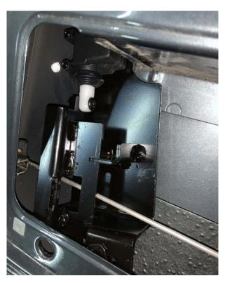
Adjust the bracket assembly to appropriate position, test the locking function. Then reinstall the cover plate on tailgate.
