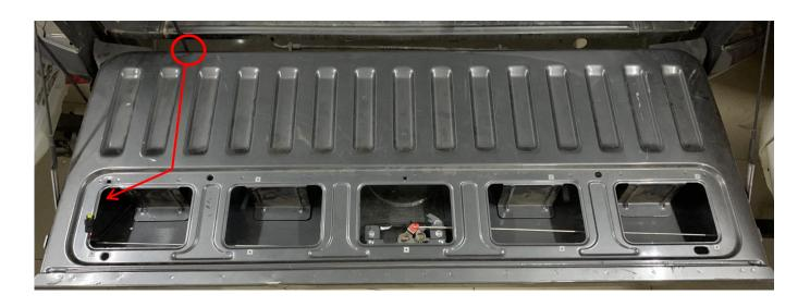
Connect the wiring to the ③ actuator
