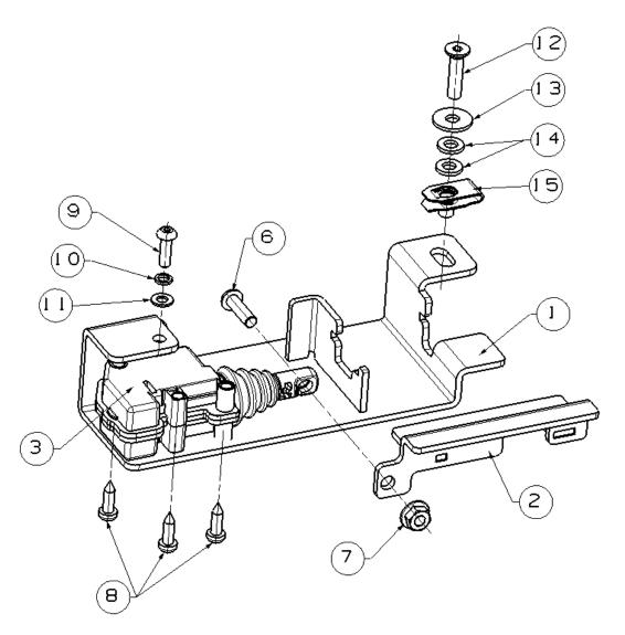
As below photo shows, install ① bracket 1, ③ actuator ⑤ Clip Nut M6 with ⑧.
