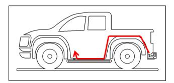
Run the wire harness from tailgate to fender flare through chassis.
