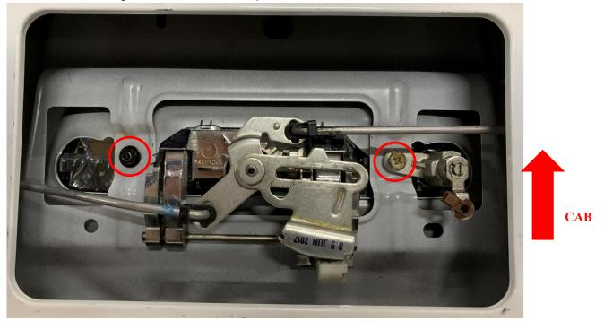
Install the bracket assembly into the tailgate, fasten it with the two original screws mentioned above. Install 3 bracket 3 and fasten it with 8 9 1:
