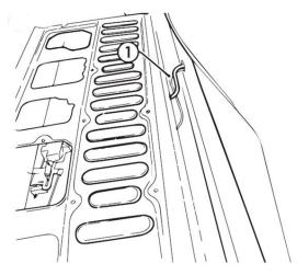
2. Route the wiring harness along the chassis rail to the following location entering the cabin via the gromet located under the rear seat.
