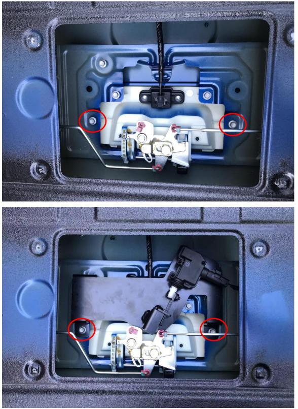
5. After installing the product, pay attention to check whether there is any looseness, move the ② with your hand, and observe whether the movement is smooth. After the check is correct and connect the wire please install the metal cover back to the tailgate in turn.
