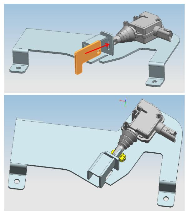
Remove the steel cover plate on tailgate by loosing the screws, and then remove the metal cover
