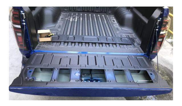
4. Remove the 2 screws of the original car, put our product into the tailgate, then install it with the removed 2 screws
