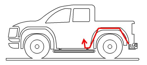
3. After routing the wires into the cabin, remove the B pillar trim panel to locate the wiring harness plug and find the Green wire & Red wire as shown in the picture below. Splice and attach the tailgate central locking wiring harness.
