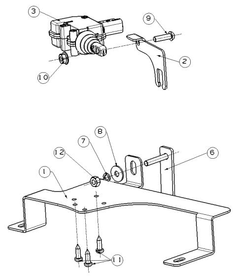
Installing Bracket, refer to the diagram above, Combine ① Bracket、② Lock catch、③ Actuator with ⑥Hexagon Socket Button Head Screws M6\_20、⑦Hex flange nut M6 and ⑧ Phillip tapping screw ST4.8\_16. Finished as the diagram shows below.
