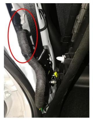
Unplug or test the wires directly to locate the signal wire in the OEM harness for the central locking lock & unlock function. Using a test light or multimeter, the desired wire will light up momentarily when the unlock/lock signal is pressed on the key fob.
