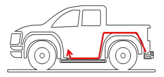
Remove B Pillar trim cover and locate the harness as shown
