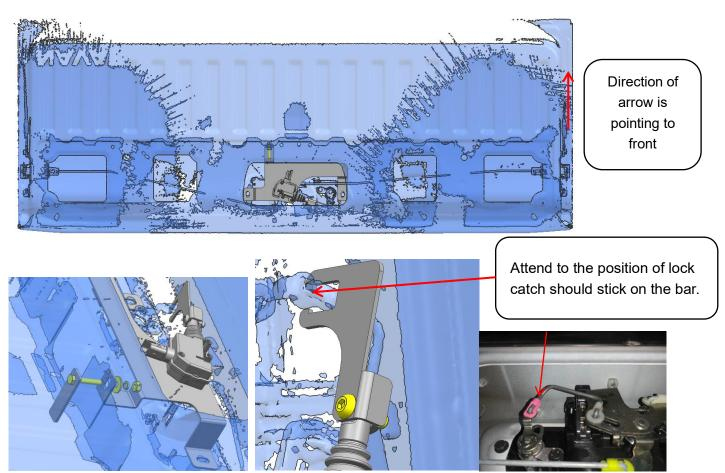
Install the steel cover plate back to the tailgate after the installation, wiring harness connection and testing. The ways of wiring harness connection show below.
