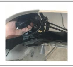
c. Connect the T-shaped clamp to the front edge of wire harness.Fix it with plier.
