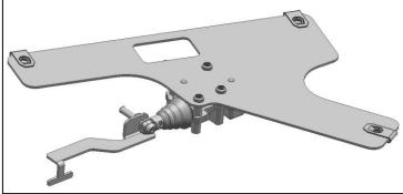
Then install the bracket inside of tailgate, fasten it with 7 ® 9
