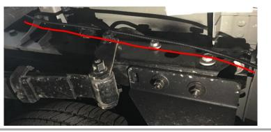
Disassemble fender flare by loosening the plastic screws.
