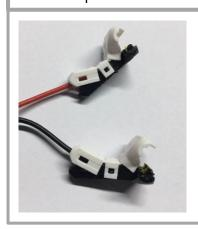
**d.** Then connect the T-shaped clamp with original actuator wire harness. Red wire connects to grey-brown wire (original wire). Black wire connects to purple-green wire. (Original)
