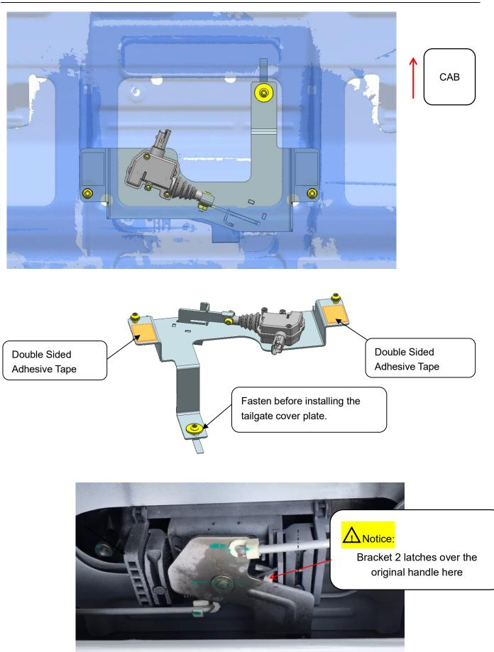
For easier positioning of the bracket, you will have to undo the 2 torx bolts that hold the tailgate handle in place. Once both ends of the bracket has been placed inside the tailgate, you may slide it 4/6
