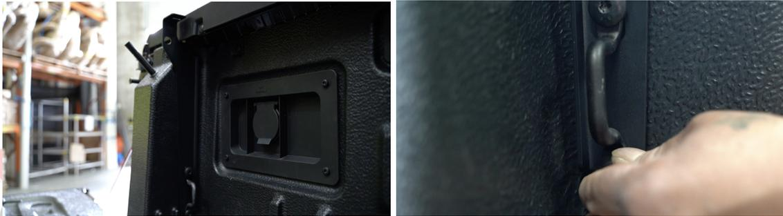
13. Remove the two side-by-side plastic clips using a screwdriver and a trim removal tool. Place the rectangular spacer in the recessed part of the tub rail, then place the L-bracket on top. Use the long M6 allen key head bolts, spring washers and washers and hand tighten the bracket. Repeat this step on the other side.
