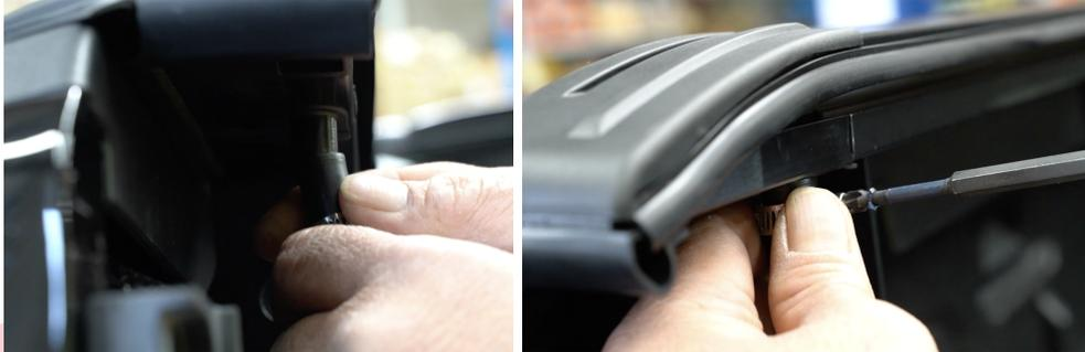
21. Plug in the harness to power the roller cover if you have an electric roller & remember to place the fuse back in the fuse holder.
