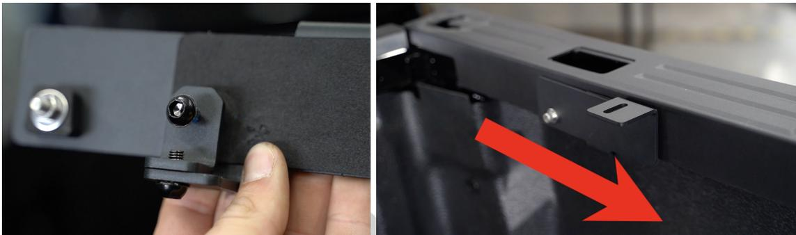
15. If you have an XLT or wish to install the XLT sports bar, make sure to place some foam tape over the holes where the sports bar used to mount, to ensure no water or dust gets through.
