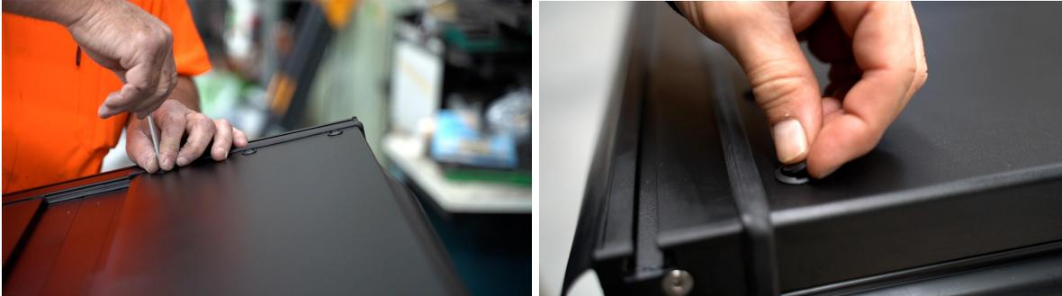
5. Now that the top cover is in place, tighten the M6 flange bolts that hold the roller cover arm together.
