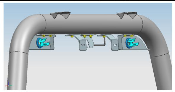
3. Install and tighten the camera on the holder shown as below.
