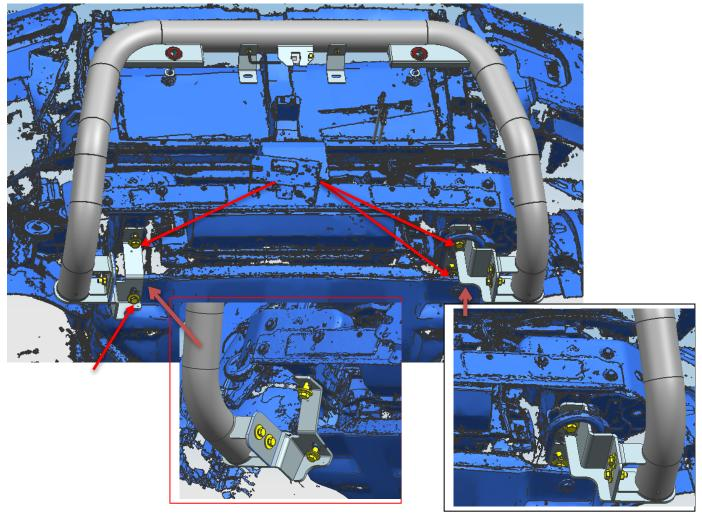
7. Install the license plate on the support bracket shown as below.
