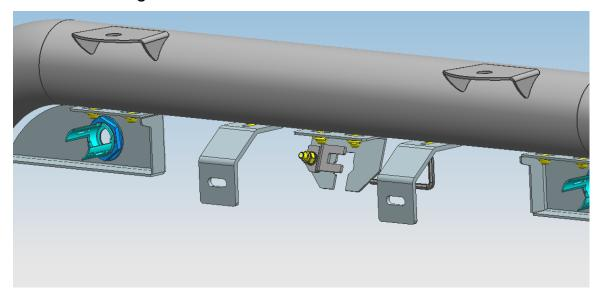
4. Put the radar inside the radar hole then tighten by hardware shown as below.
