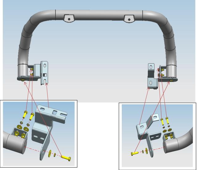
2. Install support bracket, sensor brackets and camera holder on the nudge bar by hardware shown as below.
