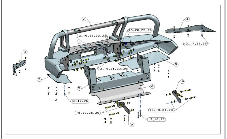
Step 1: Install the (5) winch frame on vehicle as above picture. You can install the winch now if you need.
